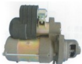
M93R3035SE 24V/6.0KW/10T Weichai Deutz: TBD226B
