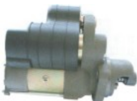
M93R3025SE 24V/6KW/10T Dongfeng Commins: ISDe
